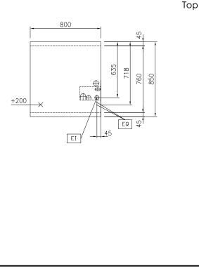
Modular Cooking Range Line thermaline 85 - 4 Zone Electric Solid Top on Warming Cabinet, 1 Side with Backsplash H=700 The company reserves the right to make modifications to the products without prior notice. All information correct at time of printing.
